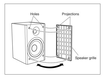
To remove the speaker grille, insert your fingers around the projection at the top of the speaker grille, then pull gently towards you while holding the side.
